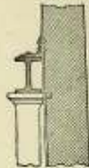
Fastening of the Sheet Iron Casing at -- B-- and support of blastpipe.
