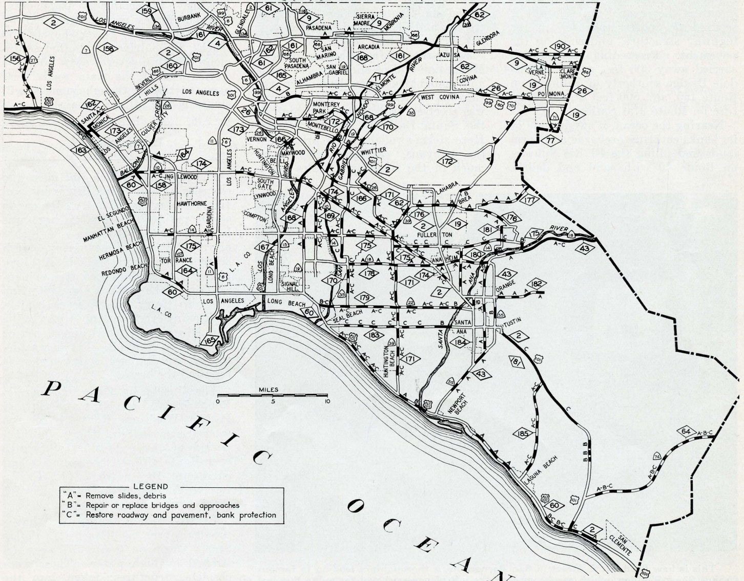
Locations of State Highway damage in Los Angeles, Ventura and Orange counties marked by black blocks on roads. Legend explains necessary restoration work.
